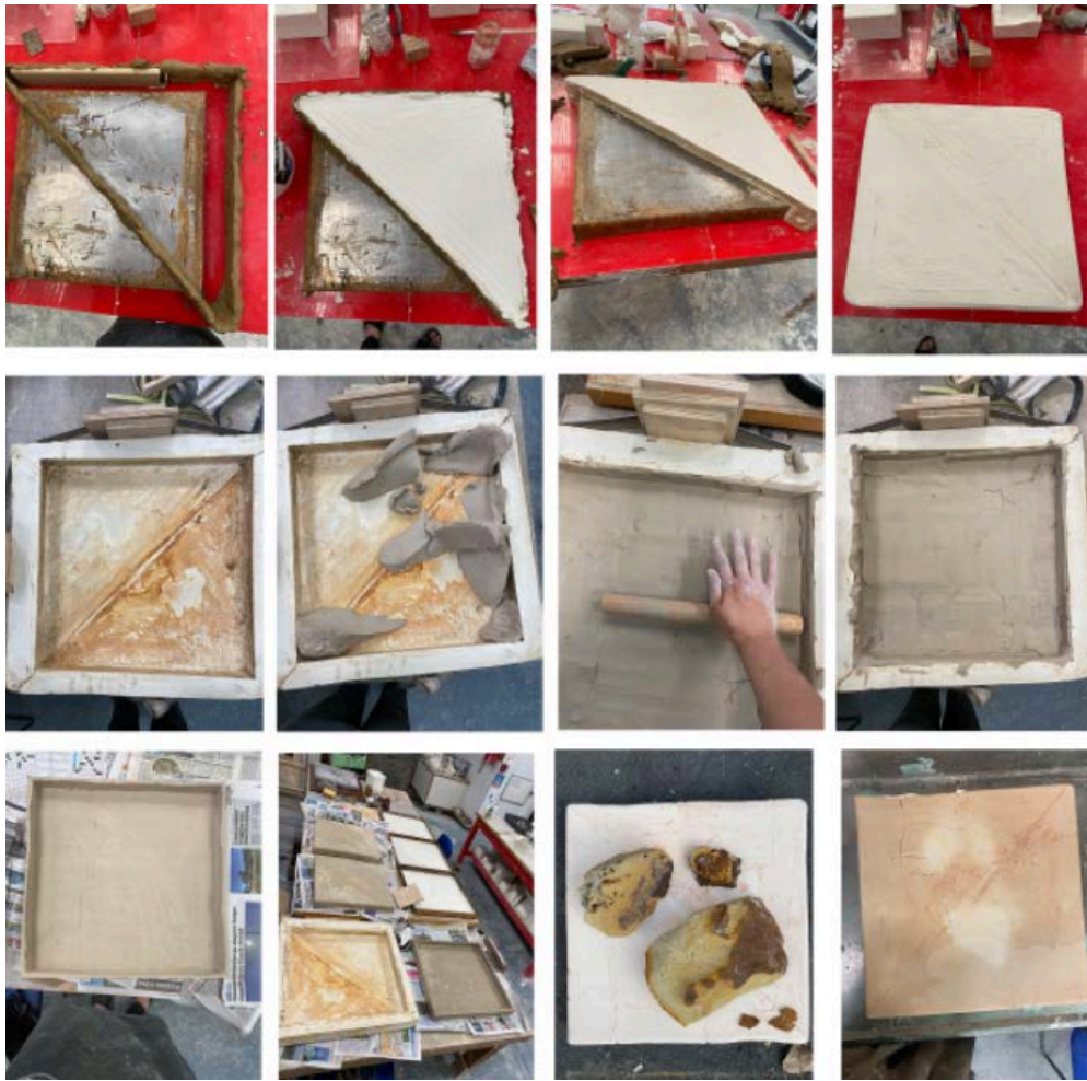
Figure 87-90, Process photo of making a mould of steel tray , Michaela van der LAAN, 2022
