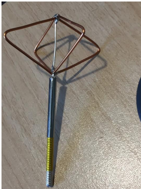
Figure 11. Finished, Constructed antenna without end plug. By Brennan Mair, 2020
