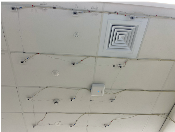
Figure 3.2: Sensors placed on ceiling of test room
