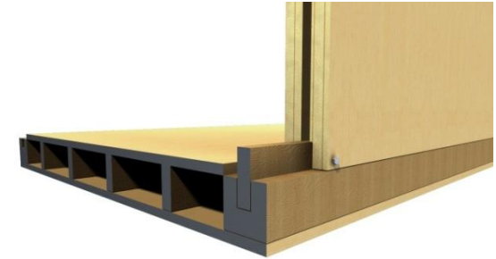
Figure 19- Floor Element to Wall Panel Connection
