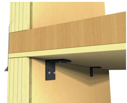
Figure 20- Intermediate Floor Connection
