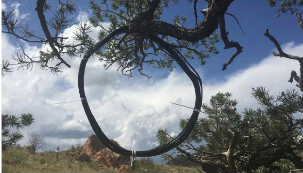
VLF Receiver made from eight-core signal cable and secured with cable ties by composer and media artist Thomas Rex Beverly, Ohio, USA
