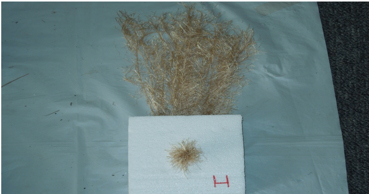
Figure 2: Artificial roots created by attaching bundles of polyester threads to the under-side of the polystyrene pad.
