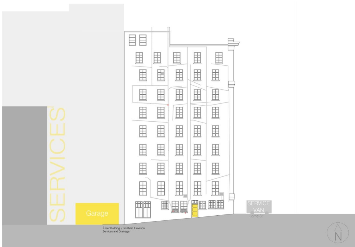
Figure 5.3.2: Diagram of Lister Services, Access Points (Yellow) and Inspection Junctions (Red)
