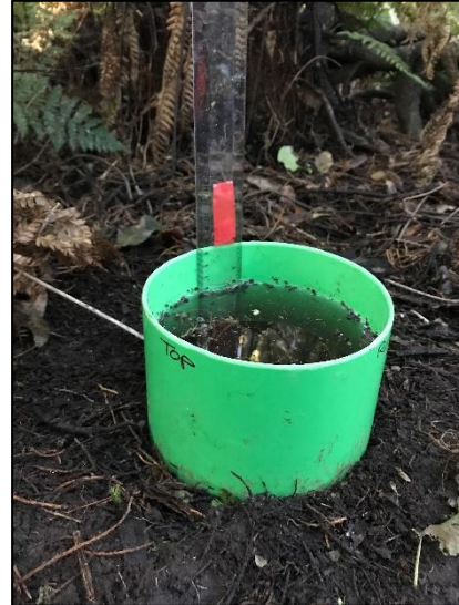
Figure 3 Infiltrometer Filled with Water and Ruler to Read Water Level
