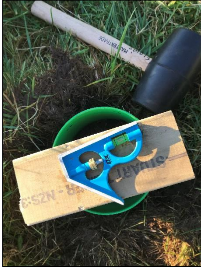
Figure 4 Levelling the Infiltrometer to Ensure Even Water Levels
