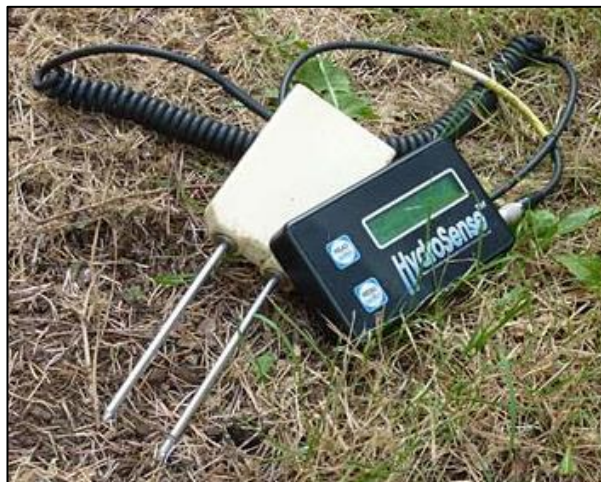
Figure 1 TDR device used for soil moisture measuring
