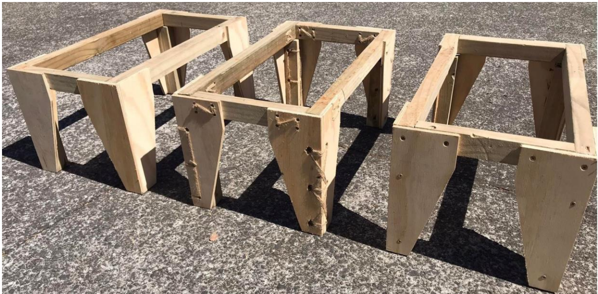
Figure 39: Three different table frames with three different types of assembly (Chemical-wood glue, Lashing-string, Mechanical-screws)
