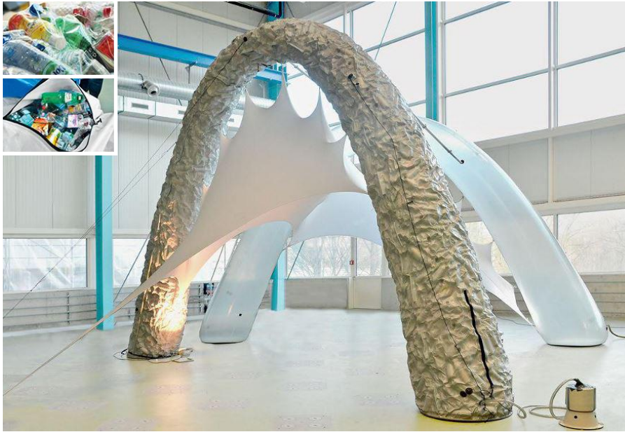
Figure 4: Arch structure using empty plastic bottles
