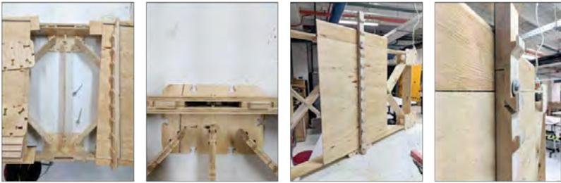
Figure 1. Early Stage ‘mock-up’ tests (from left to right: Frame Parts (tolerance test), Structural Cavity Batten Fixing, Rigid Air Barrier Testing, integrated weatherboard fixing).
