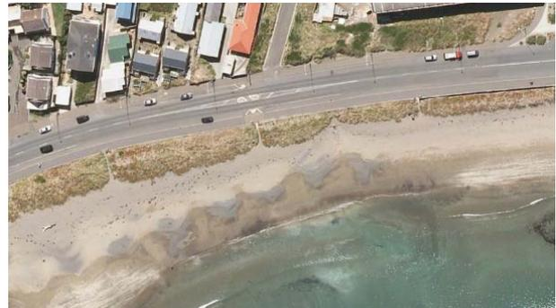
Figure 9 An aerial perspective of Lyall Bay showing the straight access pathways and an example of the erosion cut caused by discharging stormwater above the high tide mark. Paths through the dunes can also be seen; foot-traffic damages dune plants and so reduce resilience of the dunes.
