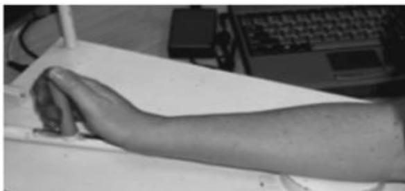
The participant was seated in a comfortable chair, while his/her hand rested on a special handle and lever, which, in turn, was able to revolve around a vertical axis. The fulcrum of the rotating segment was treated as the upper third of the forearm. In this position the forearm and wrist could perform abduction and adduction.
