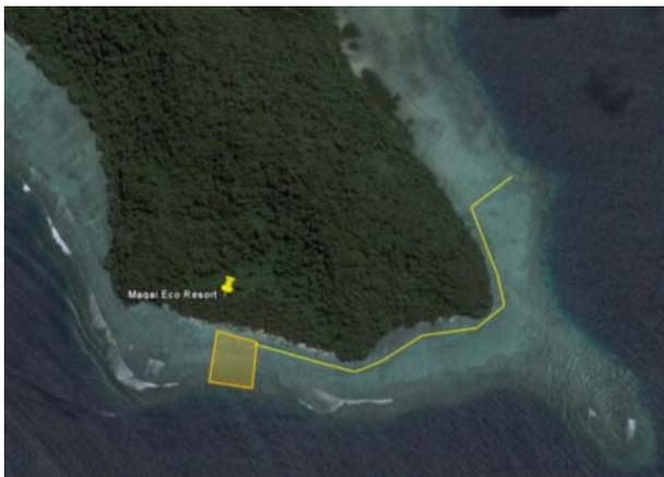
Figure 3. Access for Maqai at high tide is across the reef (100 m wide area – orange box), and at low tide from the mooring to the east (750 m – yellow line). (Source, Google Earth).
