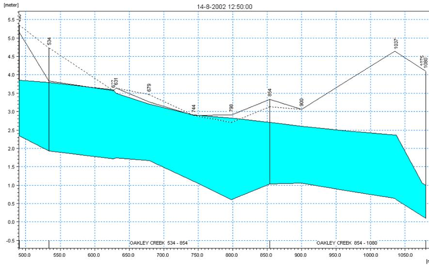
**Figure 6:** Longitudinal section of the downstream end of the creek.
